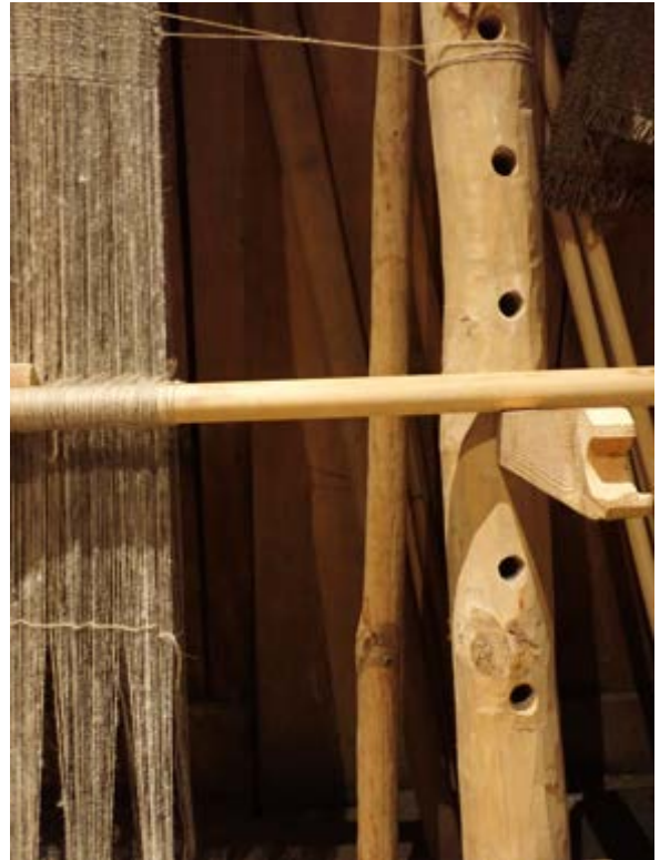
The pole holders could be adjusted by placing them in different holes as the weaving progressed down the loom.
