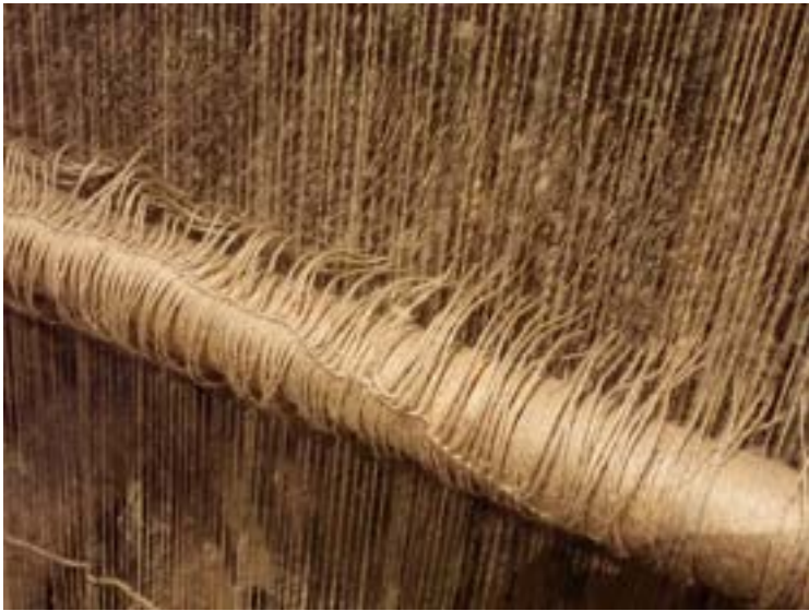
The warp threads at the back of the loom were tied to a pole so that they could be moved forward to create a shed and then released to create a shed with the opposite warp threads.
