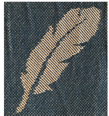
Example of split-shed weaving: straight twill feather with broken twill background woven in 3/2 cotton (Rachel Abbott)
